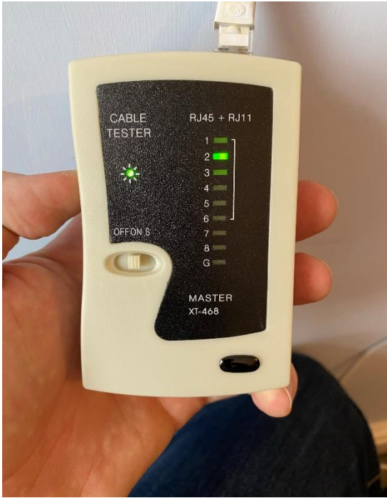
Cables are now tested using a cable tester.
