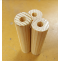
Second collection of dowels were 20mm diameter which matches the width of the arms made. These should be perfect once cut to the right length.
