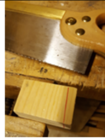
Cutting the base block using a Tenon saw.
