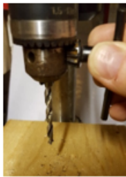
Locking a bit into the chuck with the chuck key
