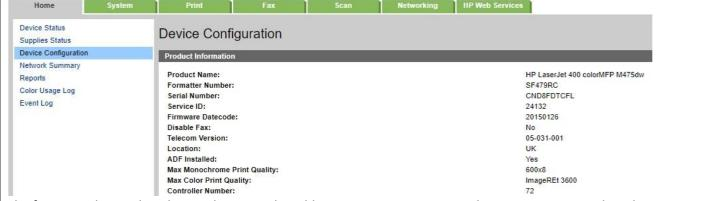
The firmware date code indicates that it is vulnerable to a JetDirect SNMP JetAdmin Device Password Disclosure exploit. Date code version 20191105 has been released to remediate this issue.
