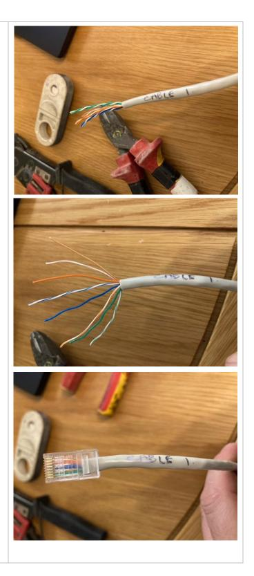
Cable 2: short across wires inside one RJ45. Produced on blue cable and labelled '**Cable 2**'.
