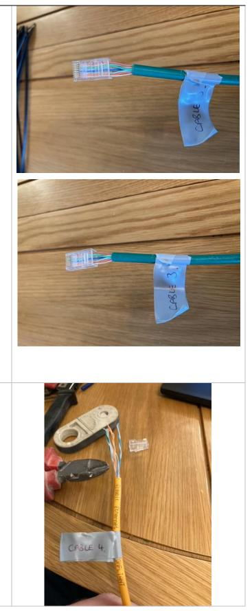
Cable 4: one RJ45 has been wired 'upside down' but has not been crimped.
