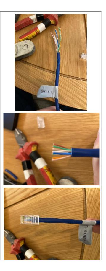
Cable 3: outer sheath of cable not gripped by crimp within one RJ45.
