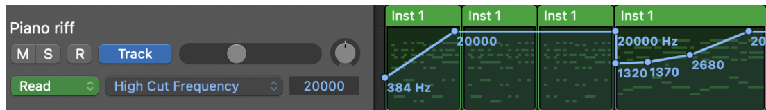
Automating low pass (high cut) frequency on piano – B section dropped again to move back in mix.
