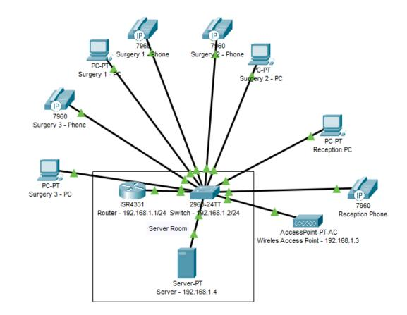
The network will use DHCP for client devices. All hardware with a label stating its IP will be set statically. The server will be configured as the DHCP server.
