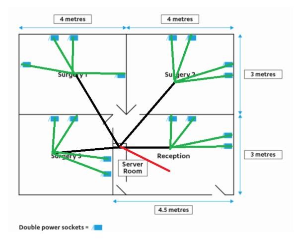
Black lines represent 8 cables in a run, green lines represent 2 cables in a run and red lines represent 1 cable.
