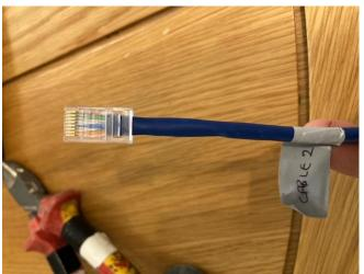
Cable 3: outer sheath of cable not gripped by crimp within one RJ45. Removed the end on the green cable and replaced – then labelled 'Cable 3'
