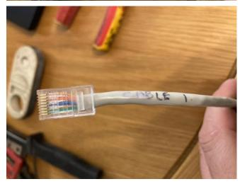
Cable 2: short across wires inside one RJ45, replaced end and labelled 'Cable 2'
