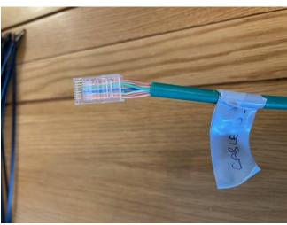
Cable 4: one RJ45 has been wired 'upside down' but has not been crimped, pulled off, replaced RJ45 and crimped. Then labelled 'Cable 4'
