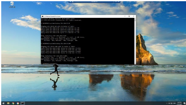
Ping test results between a wired desktop and a wired server
