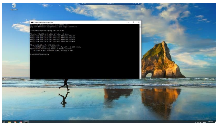
Ping between desktop (wired) and printer (wireless)
