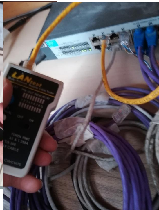
Test 2: Connectivity between patch port 2 to wall port 2
