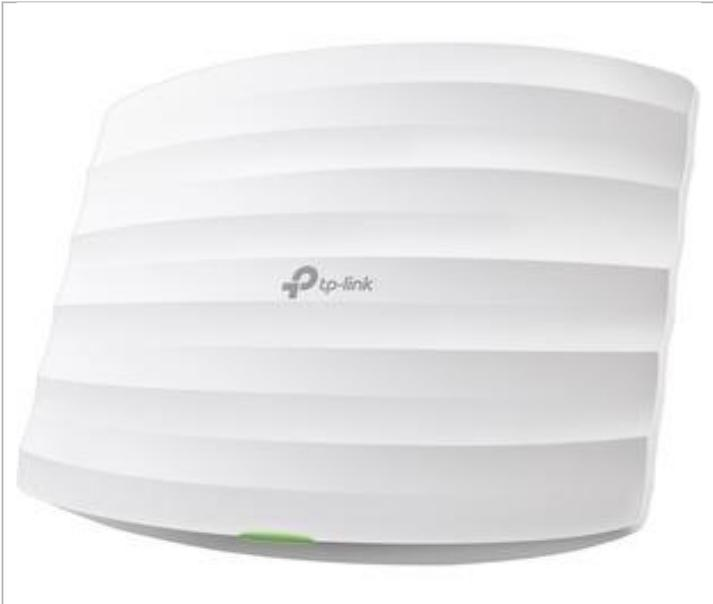
A white, cylindrical wireless access point with a TP-LINK logo on the front. It has a green LED indicator light at the bottom. | <p>TP-LINK EAP225 V3</p> <p>IEEE 802.11ac</p> <p>1.17 Gbit/s Wireless Access Point</p> <p>5 GHz, 2.40 GHz</p> <p>1 x Network (RJ-45)</p> |
